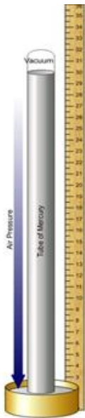
Air pressure can be measured using a simple wet barometer as shown.
