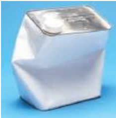
This metal can has imploded as the gas inside is cooled.
